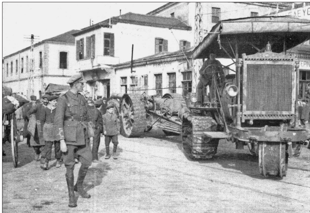
Fig. 5: Holt caterpillar tractor towing a six-inch gun, the sort of heavy equipment which blocked the main roads in the British retreat during Operation Michael, 21 March–9 April 1918. CIWM Q 31595. © IWM
